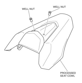
4. Clean the surface of the area shown using an isopropyl alcohol.
