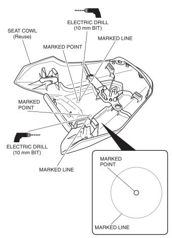
3. Install the well nuts as shown.
